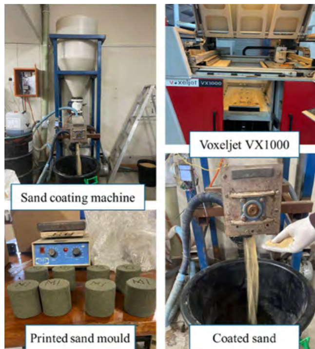
Laboratory equipment and materials used in this study included the sand coating machine, coated sand, printed sand moulds and 3D printer.
