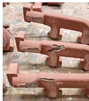
Fig. 8. Cracked cores after drying
